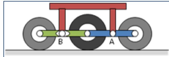
Figure 3 – Basic schematic of Linked-Bogie frame (Side view)
